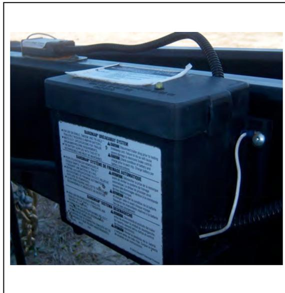
Connect the pullpin lanyard to the tow vehicle so that the pullpin will be pulled out before all of the slack in the safety chains is taken up (see Breakaway Brake System figure). Do **not** connect the pullpin cable to a safety chain or to the hitch ball or hitch ball assembly. This would keep the breakaway brake system from operating when it is needed.
