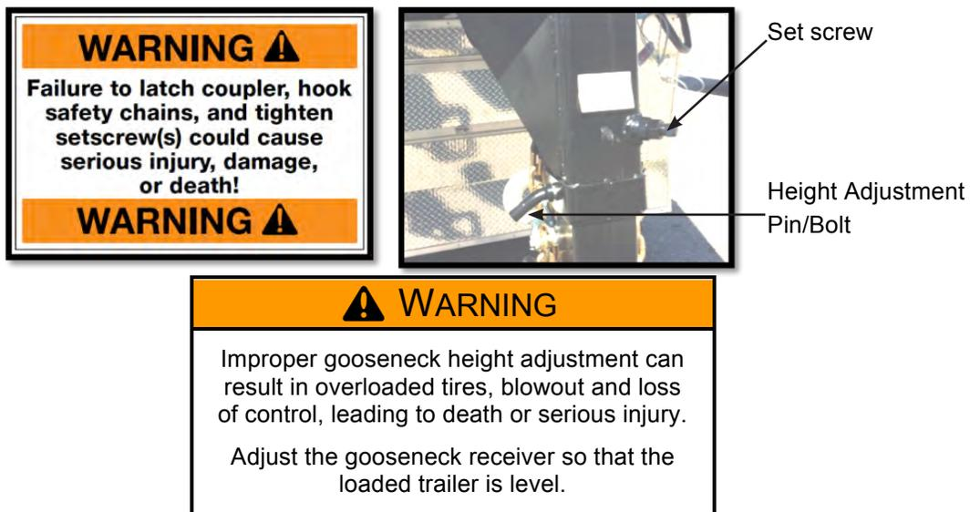
A trailer having a gooseneck hitch will have one or two drop leg jacks for raising and lowering the gooseneck ball receiver. Because several drop leg jack mechanisms are available, the general instructions below may vary slightly from the jack manufacturer's instructions.
