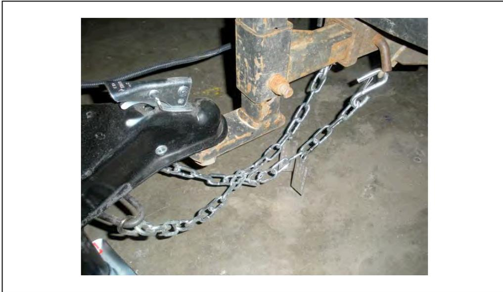
Visually inspect the safety chains and hooks for wear or damage. Replace worn or damaged safety chains and hooks before towing.
