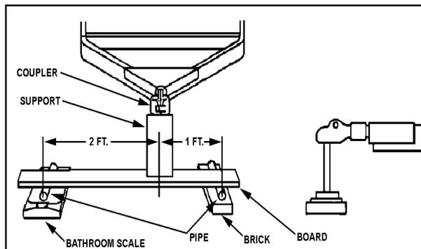
Lower the tongue until the coupler rests on the block support and the jack is ½ inch above the ground.
