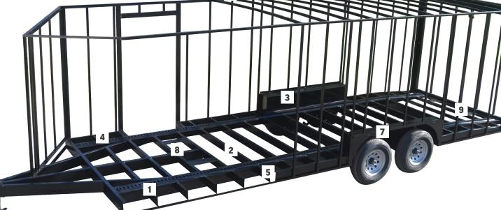
1 TUBE MAIN RAILS Lighter than I-Beam competitors while providing more torsional rigidity. Our trailers haul more and last longer.
