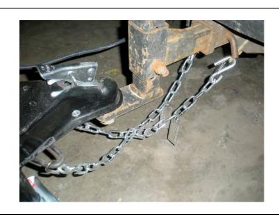
Visually inspect the safety chains and hooks for wear or damage. Replace worn or damaged safety chains and hooks before towing.
