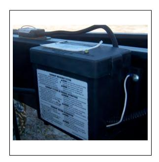
Connect the pullpin lanyard to the tow vehicle so that the pullpin will be pulled out before all of the slack in the safety chains is taken up (see Breakaway Brake System figure). Do **not** connect the pullpin cable to a safety chain or to the hitch ball or hitch ball assembly. This would keep the breakaway brake system from operating when it is needed.
