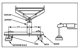
Lower the tongue until the coupler rests on the block support and the jack is ½ inch above the ground.
