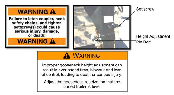
A trailer having a gooseneck hitch will have one or two drop leg jacks for raising and lowering the gooseneck ball receiver. Because several drop leg jack mechanisms are available, the general instructions below may vary slightly from the jack manufacturer's instructions.
